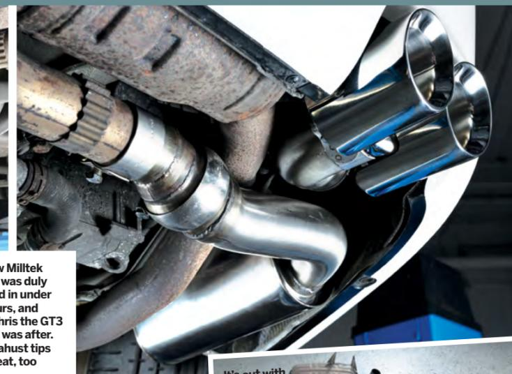
system with a fair amount of ease – not even having to take off the rear bumper – and within about two hours the shiny new Milltek was fitted. At this point I should mention that all Milltek Sport systems simply accept your original OEM tailpipes, which is great, but as mine were looking a little tired I contacted Design911.com and got my hands on some new tailpipes, which had a slightly more aggressive look and filled the outlet surround much better, too.
