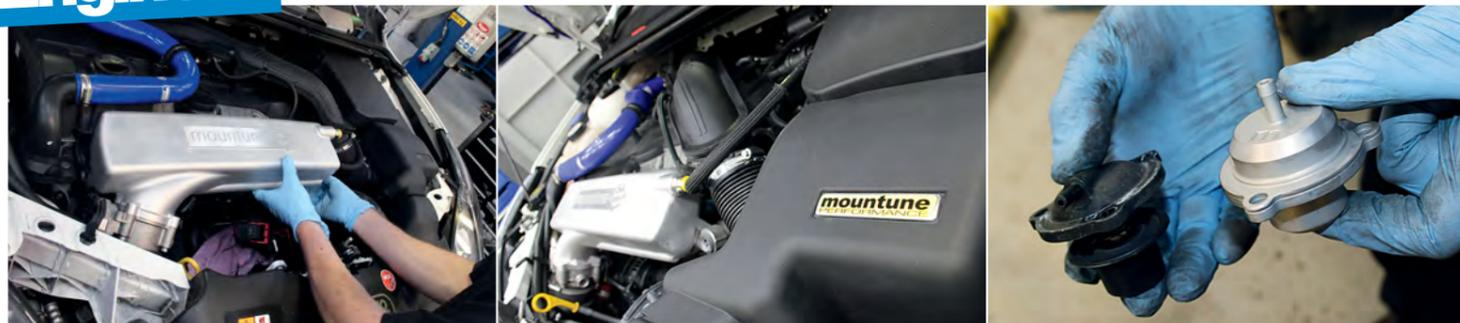
Mountune inlet, air box and recirculating valve are all part of the MR375 kit
