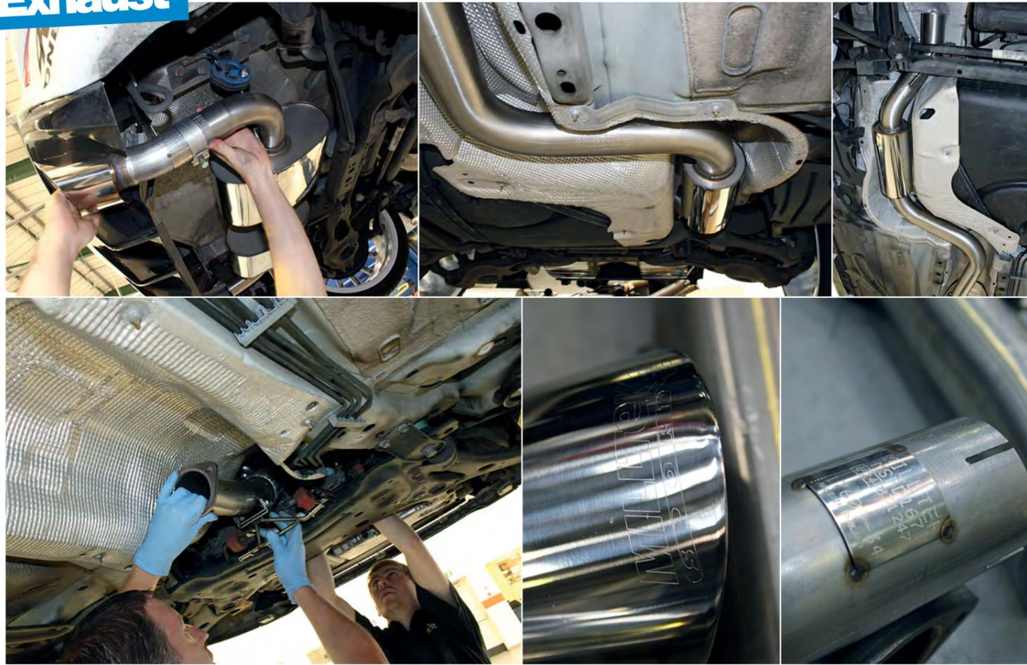
With the uprated fuel pump fitted, Mountune's technicians could offer up the new Milltek exhaust into place
