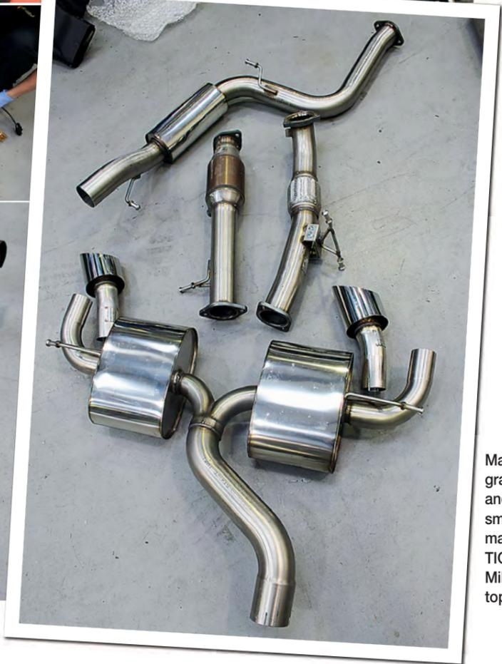
Made from aircraft-grade stainless steel and featuring smooth radius mandrel bends and TIG-welded joints, Milltek exhaust is top notch
