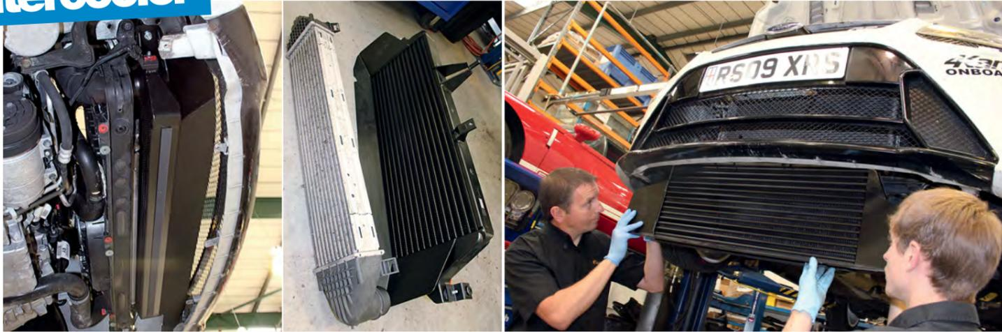
Mountune designed Pro Alloy intercooler slots neatly into place. It's built to very high standards and is a fair bit larger than the original RS item as you can see
