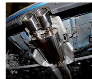
**Short flexible section at front of exhaust system (below, right) allows engine a degree of movement without fracturing pipework. Catalytic converter is incorporated in high-flow downpipe. Tailpipe can have twin outlets, as here, or larger single pipe for about £20 more**
