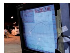
**Car certainly feels like it has extra power and torque, but what would the rollers tell us? Thanks to the Scooby Clinic near Chesterfield we were able to find out for sure: in fact, power peaked at 203.4bhp, torque at 215lb/ft - and that all the way from 2400 to 4500rpm**
