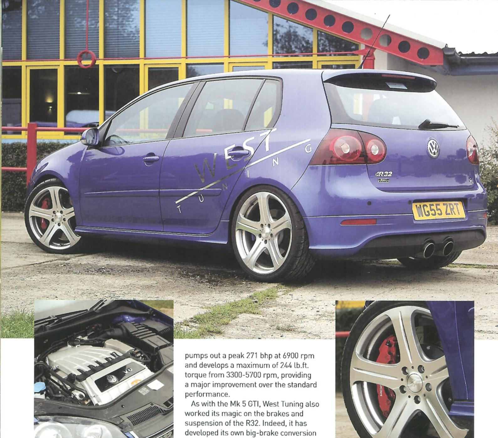
the internal diameter by about 10 per cent and reprofiling it to improve its induction ability. He also installed a fulllength free-flow Milltek Sport stainlesssteel exhaust system, incorporating high-flow catalytic converters. Not only does the Milltek system allow the engine to breathe more easily, but it also gives it a beautiful engine note, even more purposeful and sonorous than the standard system, without any of the loud, rorty noises so commonly associated with big-bore sports systems.
